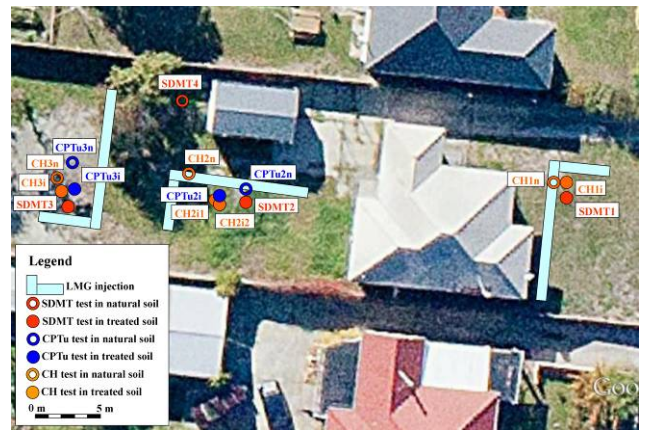
Fig. 13. Site investigation and RAP works realized at 121 Bower Avenue.
