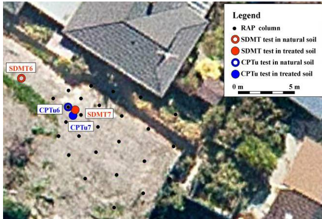
Fig. 7. Site investigation and RAP works realized at Site 4, RAP Spacing Trial Area 1-2 – Avonside Drive.
