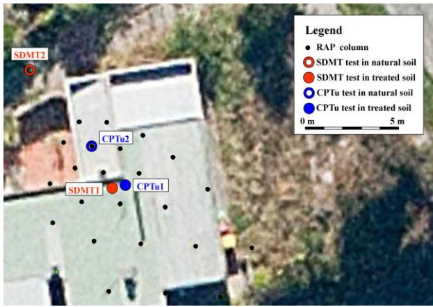
Fig. 10. Site investigation and RAP works realized at Site 6, RAP Spacing Trial Area - Wairoa Street.
